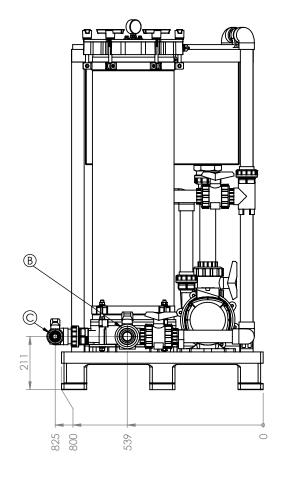
A) SUCTION, 63mm BALL VALVE. B) DISCHARGE, 50mm BALL VALVE. C) DRAIN, 25mm BALL VALVE.
